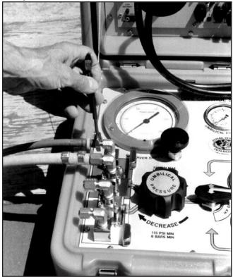
Fig. 7 Always use the right size wrench to connect the hoses to the KMACS 5.
